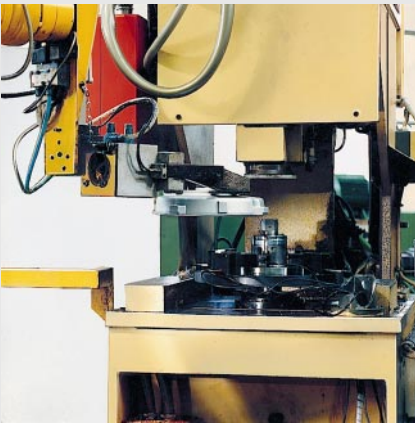
Fully automatic final check of endshields of ELMO-F and -G drives.
