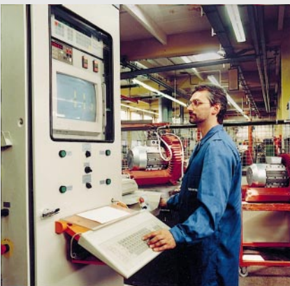
Check of performance data and printing of the test protocol.
